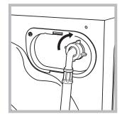
2. Connect the other end of the water inlet hose to the washing machine, screwing it onto the appliance's cold water inlet, situated on the top righthand side on the rear of the appliance (see figure).
